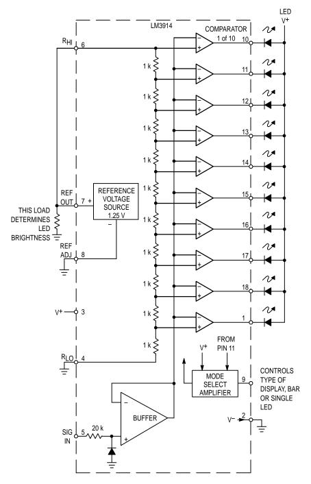
Figure 4. LM3914 Block Diagram
