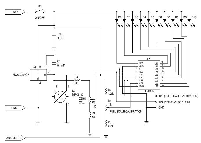
Figure 2. MPX5100 Pressure Gauge
