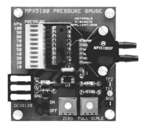
Figure 1. DEVB129 MPX5100 Bar Graph Pressure Gauge
